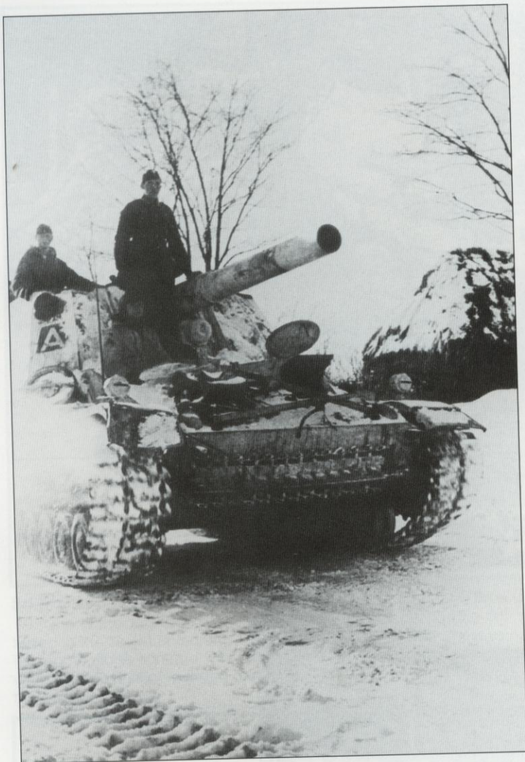
This series of three photos provides a view of a maneuvering battery of Hummel 15cm self-propelled howitzers belonging to an independent battalion of heavy artillery. All three vehicles (marked with the letters "A", "G", and "O") are equipped with wide "Ostketten" and are partly or completely camouflaged with white paint and snow.
