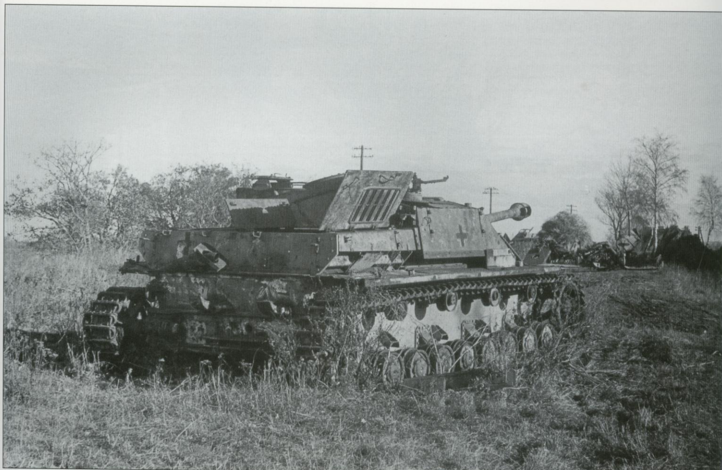
This StuG IV was knocked out during the fight for Pomerania in the spring of 1945. Note that a camouflage pattern was applied to the assault gun's superstructure while the hull was not camouflaged at all. This vehicle has a single armor plate bolted to the side of the superstructure for additional protection.
