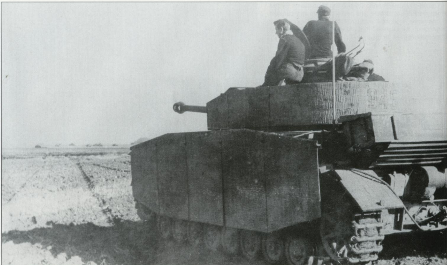
A Pz.Kpfw. IV Ausf. H with a full coat of Zimmerit anti-magnetic paste applied to its exterior. Note the non-standard stowage box added to the rear of the vehicle. By the autumn of 1943, the German Army was in full retreat. The Soviet Army fielded 2,600 tanks between Smolensk and Rostov with the intention of pushing the Germans back to the Dnieper River before the year's end.
