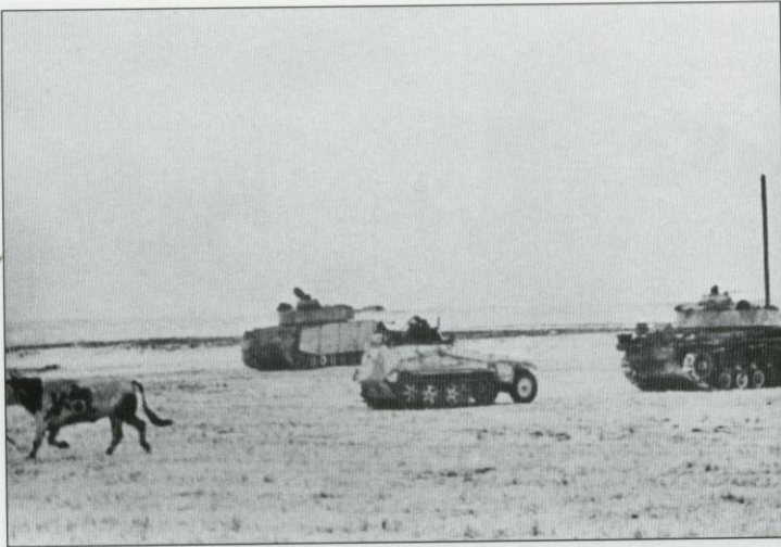
Three different vehicles belonging to a staff unit from a tank battalion roll across the frozen winter landscape. At right is the Pz.Bef.Wg. III Ausf. K, in the middle is a command model of the Sd.Kfz. 250, and in the background is a Pz.Kpfw. IV. All the vehicles are painted in winter camouflage (the bull's winter coloring is natural).
