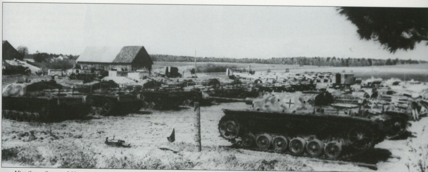
After the collapse of Heeresgruppe Nord , the Soviets collected tons of combat equipment from all around the northern areas of Russia, including these StuG III Ausf. F/8s and Ausf. Gs, which originated from the same unit. Almost all of the StuGs seen in this photo are painted in similar camouflage composed of a green and brown pattern over a dark yellow background, which is most clearly seen on the first vehicle of each row.
