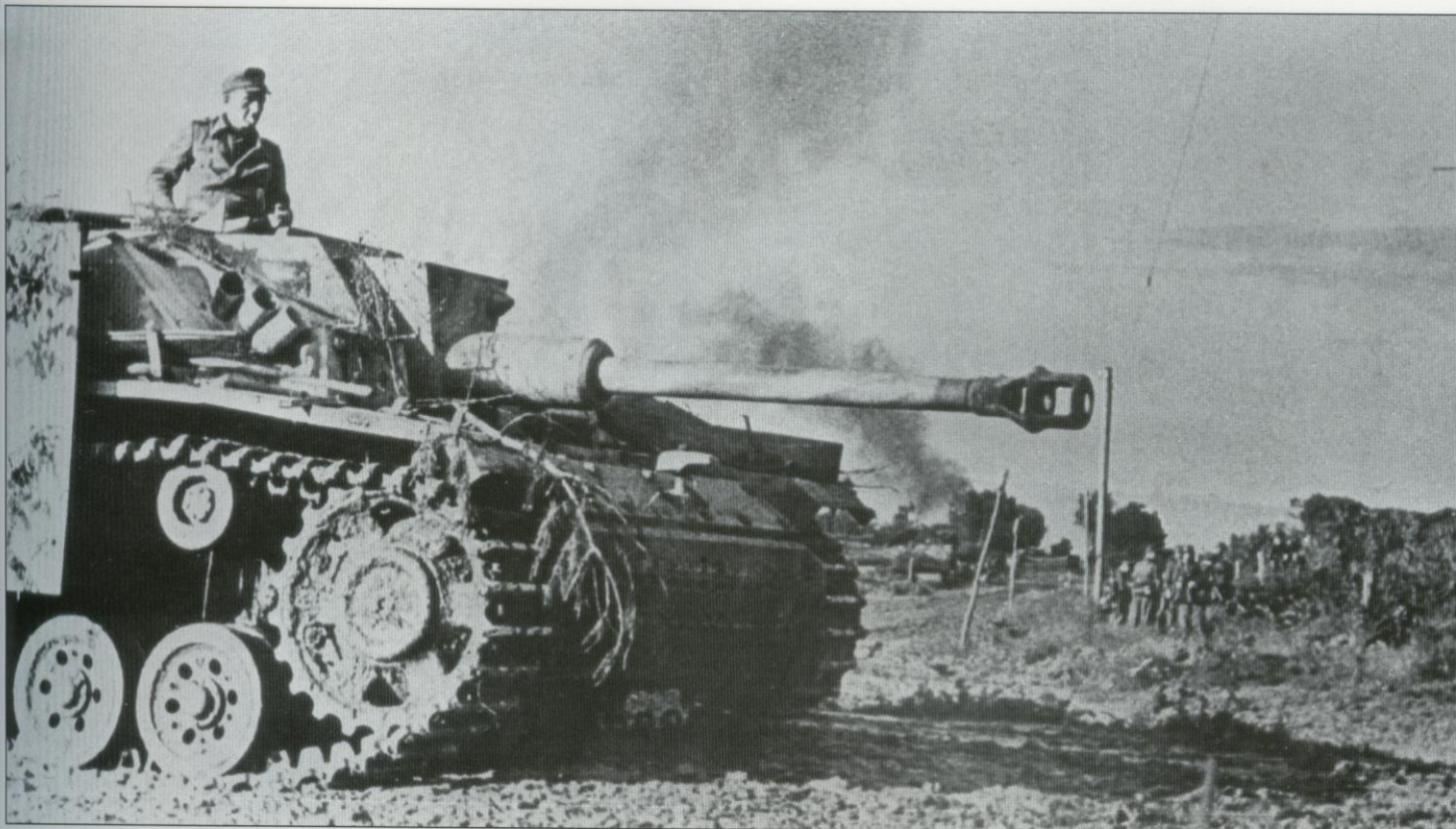
This photo shows a StuG III Ausf. G in action. The front part of the right set of skirts is missing, so the smoke grenade launchers are clearly visible. The muzzle brake illustrates the typical German practice of painting the muzzle brake of tanks and self-propelled guns a very dark color — usually dark gray. During combat in the autumn of 1943, the Panzerwaffe lost the largest number of StuGs since the beginning of war against the Soviets — about 200 vehicles per month. Most of them were lost on the Eastern Front, of course.
