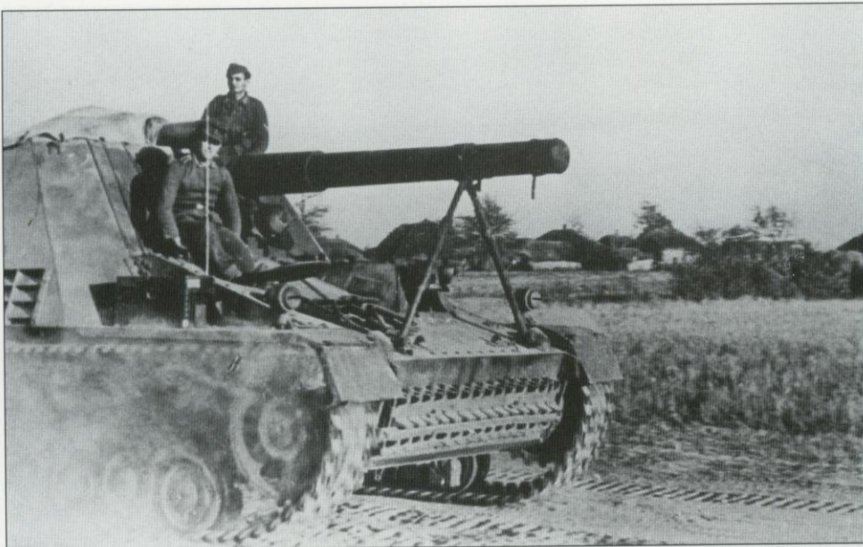
A Hummel on the march. Note how the camouflage of this self-propelled howitzer was painted on the top portions of the superstructure. As usual there is a strip of the base color paint in the area where the tarpaulin was attached on top of the vehicle.
