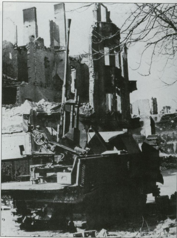
This StuG IV was knocked out during the fight for Pomerania in the spring of 1945. Note that a camouflage pattern was applied to the assault gun's superstructure while the hull was not camouflaged at all. This vehicle has a single armor plate bolted to the side of the superstructure for additional protection.
