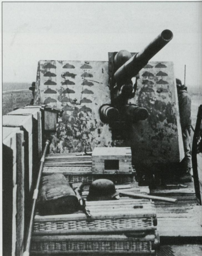
Another "88" gun from the same Eisenbahnpanzerzüge displays its successes: 26 tank "kills" on the gun shield and seven or eight air victories on the barrel. Note the damage to the right "armor plate" (composed of sand in a wooden framework), and that the gun has a dark gray barrel and a sand-colored shield.
